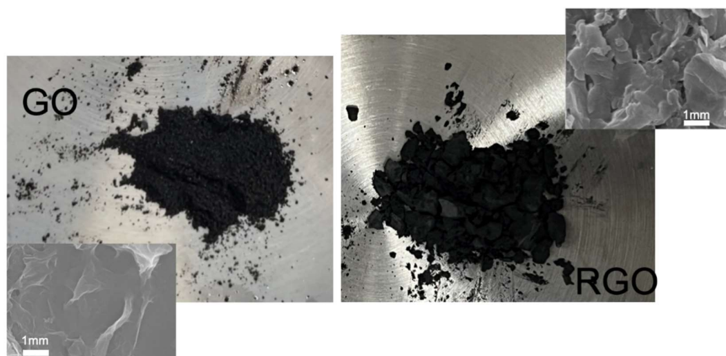
Fig. 4 Scanning electron microscope (SEM) images of graphene oxide and reduced graphene oxide
