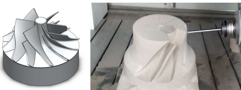
(a) Impeller characteristic model;(b) Five-axis milling of impeller sand molds
