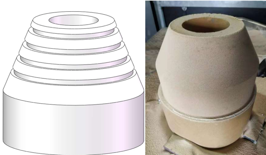
(a) Cone feature model; (b) Rotary table sand mold turning processing
