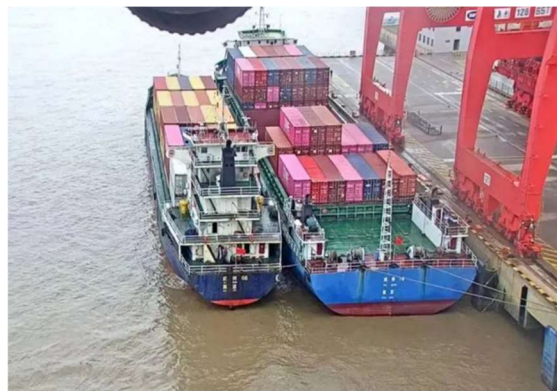
Fig. 6 Container loading and unloading operation under "double alongside berthing"
