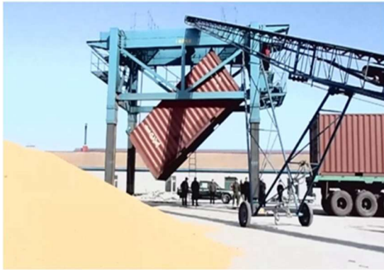
(a) mounted gantry tilting machine
