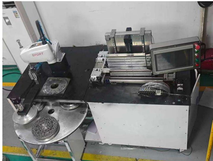
Figure 3. Physical layout of intelligent magnet insertion equipment
