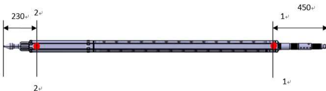
Fig. 3 Acceleration Measuring Point Layout.
