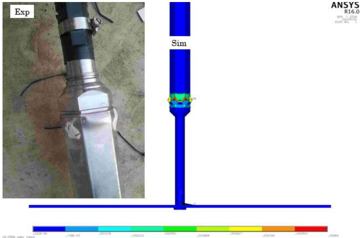
Fig. 12 Simulation and experimental results at a drop height of 4050 mm.
