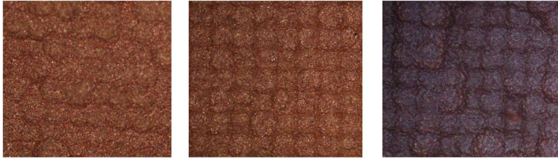
Figure 6. Optical microscopy images of double-sided electroplated copper-filled microhole arrays for Samples 5-7.
