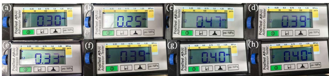
Figure 5. Adhesion strength of the composite coatings: (a) 71% CG / 29% WAR, (b) 73% CG / 27% WAR, (c) 65% DCG / 35% WAR, (d) 67% DCG / 33% WAR, (e) 69% DCG / 31% WAR, (f) 71% DCG / 29% WAR, (g) 73% DCG / 27% WAR, (h) 75% DCG / 25% WAR.
