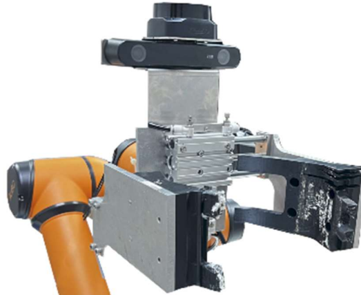
Figure 4. Experimental setup showing the AUBO-i5 robotic arm, ZED2i camera, and 2D LiDAR.
