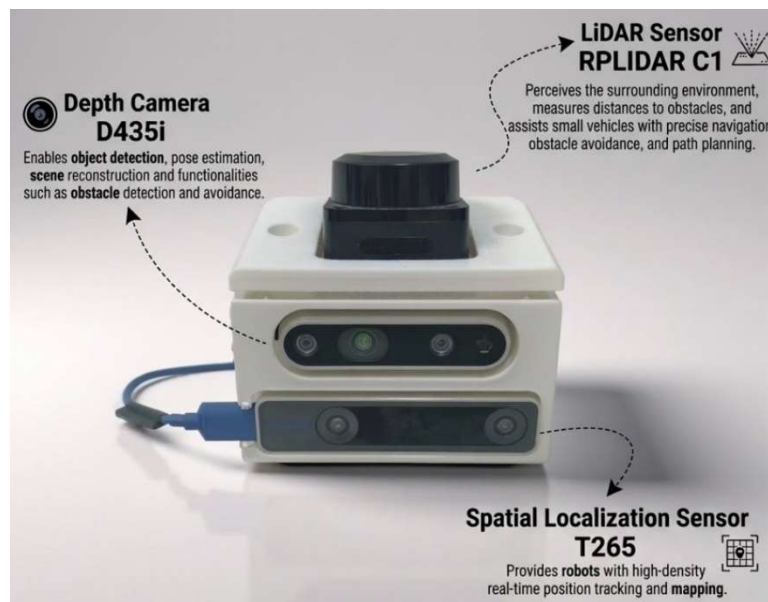
Fig. 2 Heterogeneous Sensor Fusion Architecture
