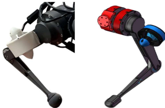
Figure 6. Design model and physical diagram of the leg-propeller integrated structure
