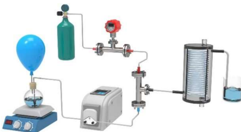
Figure 2. Schematic diagram of the synthesis of PFPE acyl fluoride in a microchannel reactor.
