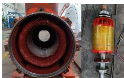
Figure 2. Partial disassembly drawing of explosion-proof motor
