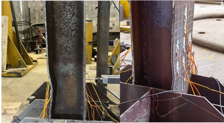
Fig. 2 Typical failure morphologies of H-section steel column specimens in different damage states
