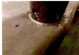
(c) Local buckling failure of the main pipe upper wall and side wall (CS-T3)
