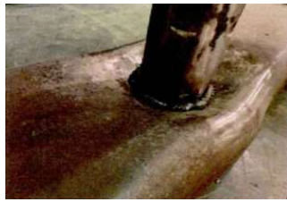
(a) Compressive branch pipe end buckling and main pipe upper wall buckling failure (CS-T1)
