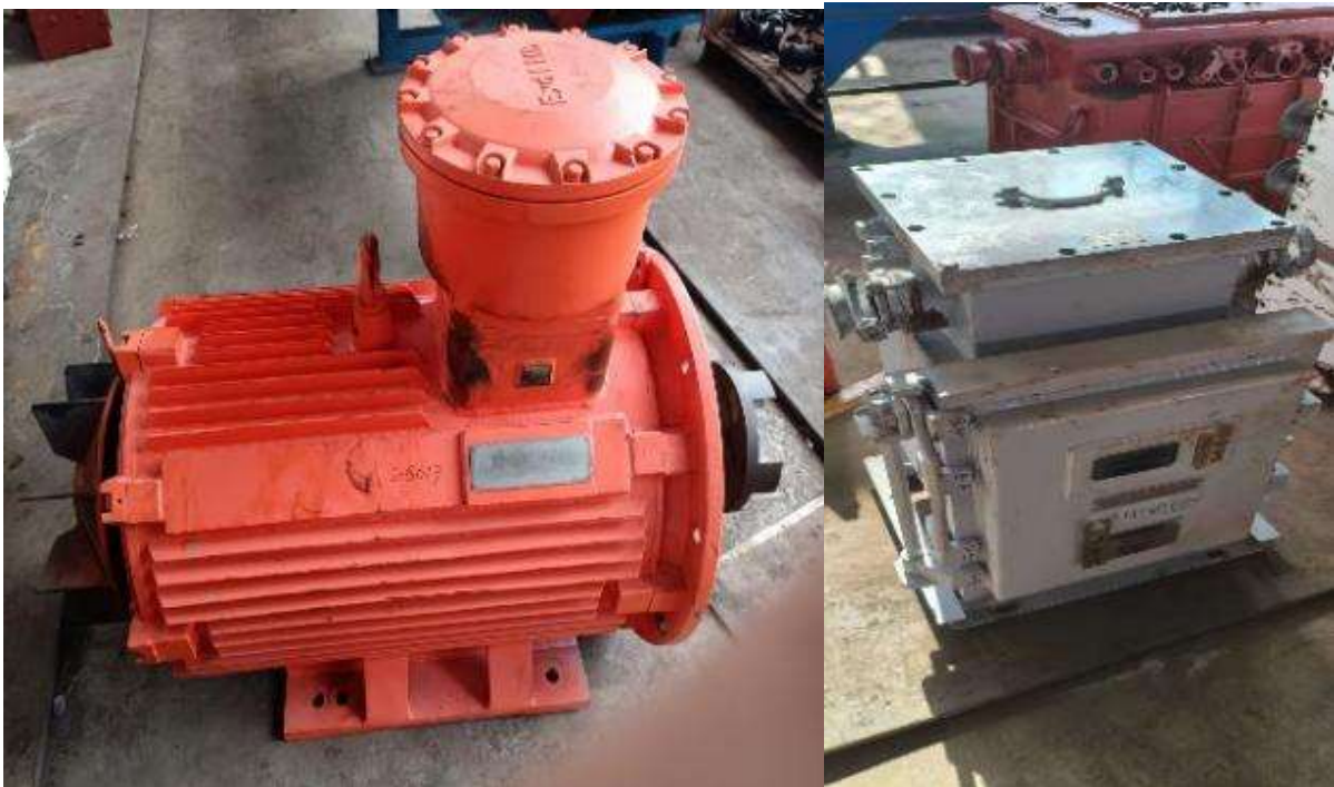
Figure 1. Physical picture of mining explosion-proof motor and electromagnetic starter
