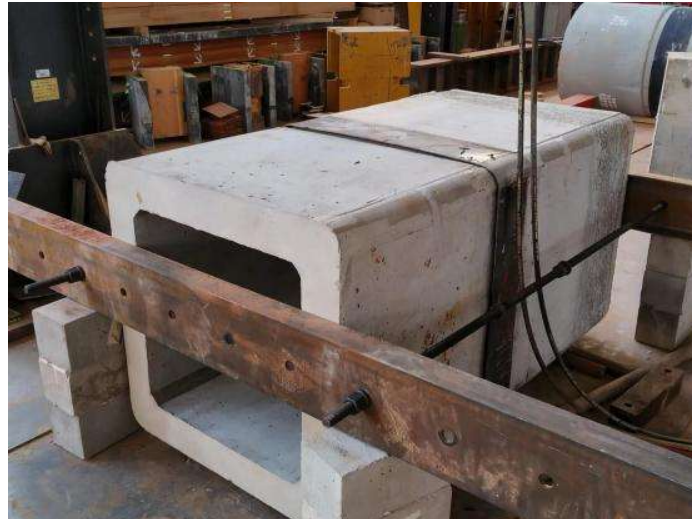
Fig. 2 Flexural test on a rectangular utility tunnel
