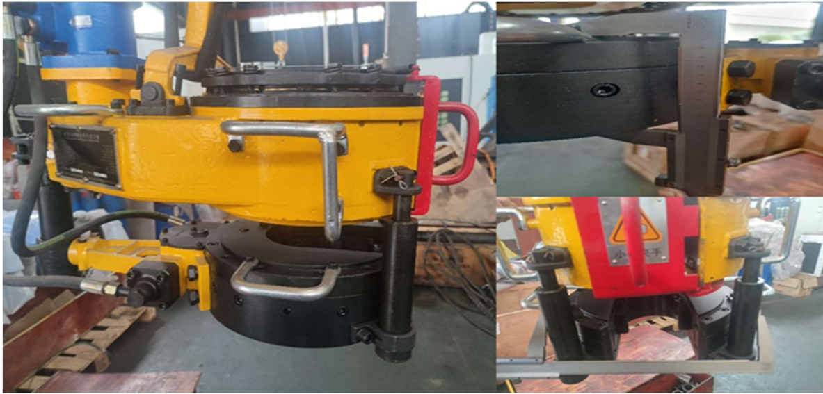
Fig. 5 Hydraulic power clamp size mapping.
