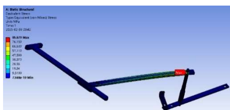
Figure 8. Stress Analysis Results of Left Linkage Mechanism
