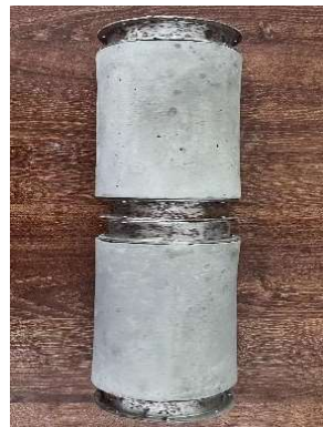
Fig. 5 The overall connection of a pair of new round culverts
