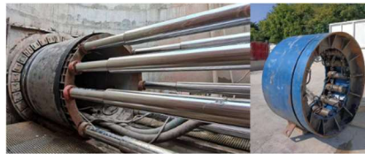
Fig. 1 Jacking cylinder and relay
