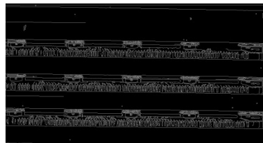
Fig. 3 Image after edge extraction using the Canny operator
