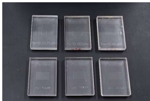
Figure 4. Physical image of multi groove template
